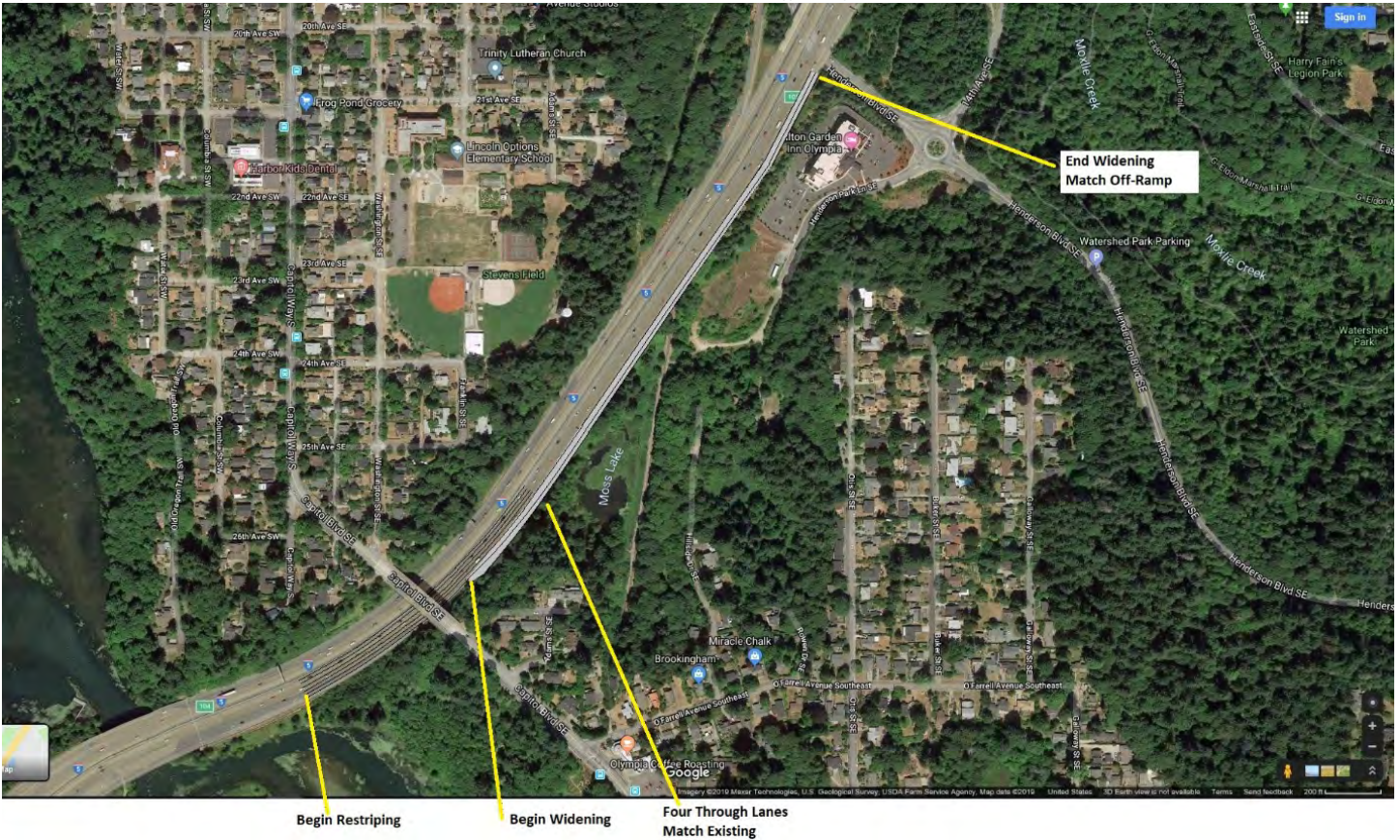
Figure 17: Northbound I-5 auxiliary lane between US 101 on-ramp and 14 th Avenue off-ramp
