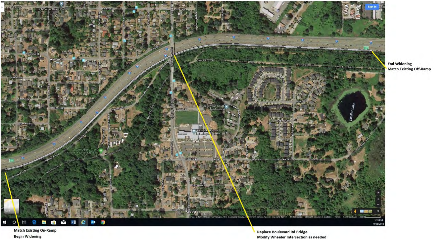
Figure 18: Northbound I-5 auxiliary lane between Plum Street on-ramp and Pacific Avenue off-ramp
