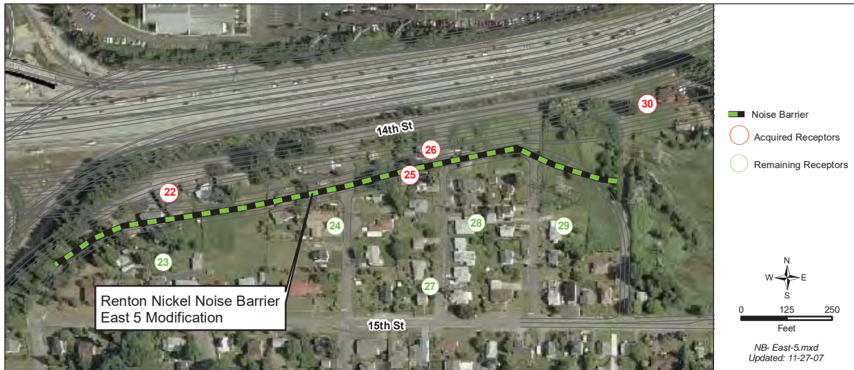
Exhibit 5-5: Noise Barrier East 5 Modification
