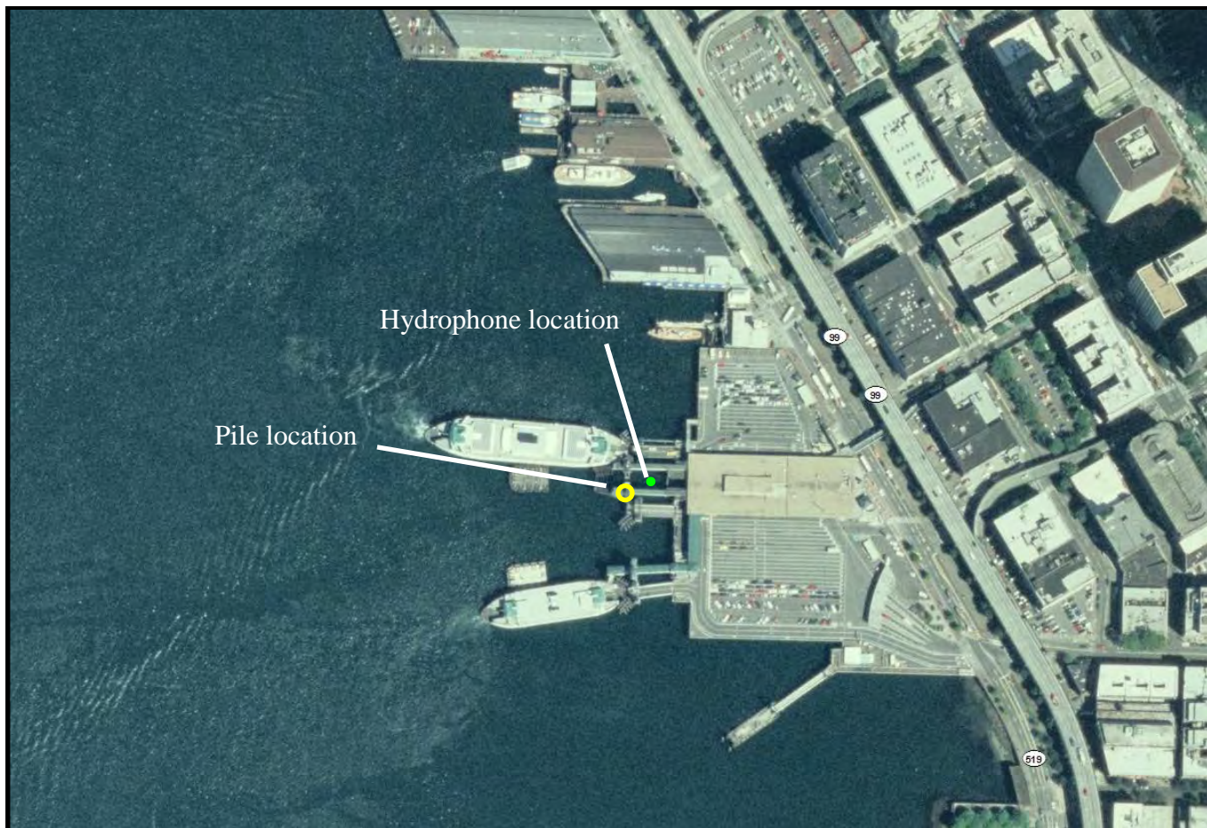
Figure 2: Approximate location of 30-inch pile and hydrophone at the Seattle Ferry Terminal Batter Pile Project.
