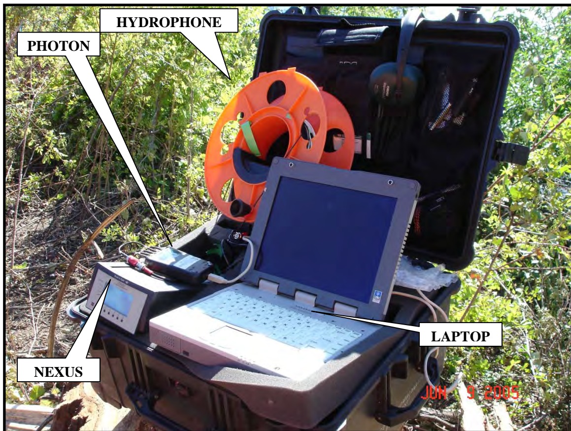
Figure 3: Near field acoustical monitoring equipment
