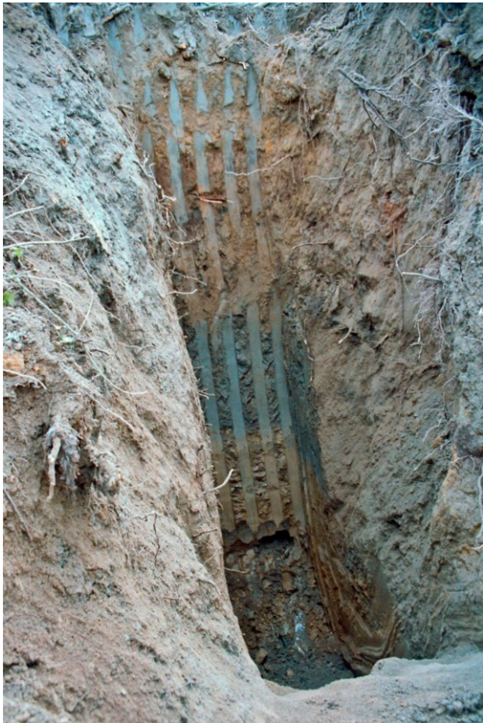
Test Pit on Beacon Hill Showing Depositional Sequence Within a Glacially Overconsolidated Clay, Paleolandslide Deposit Figure 5-4
