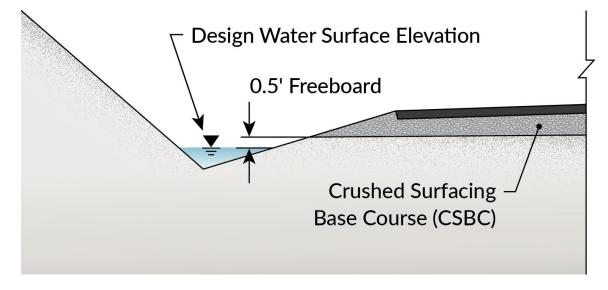
Ditches should not be confused with biofiltration swales. In addition to collecting and conveying drainage, biofiltration swales provide runoff treatment by filtering out sediment. (See the *Highway Runoff Manual* for design guidance for biofiltration swales.) Roadside ditches are to be designed so the integrity or geometry of the roadway is not compromised.
