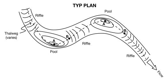
Figure 4-3 Field Slope Measurement of Non-Uniform Flow Channels Plan View
