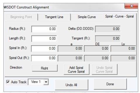
Radius - Distance from the Curve Center (CC) to the Point of Curvature or Tangency (PC/PT).
