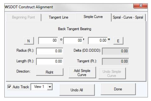
**Back Tangent Bearing** – indicates bearing from previous element or if first, can be entered similar to Bearing & Distance tab.
